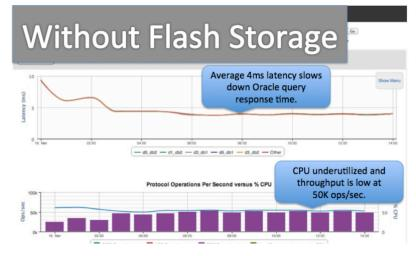
Figure 6: Oracle impact on storage without Flash
