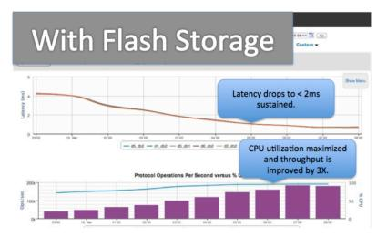
Figure 7: Oracle impact on storage with flash
